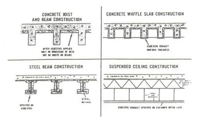
Figure 9-2 Types of Ceiling Construction
